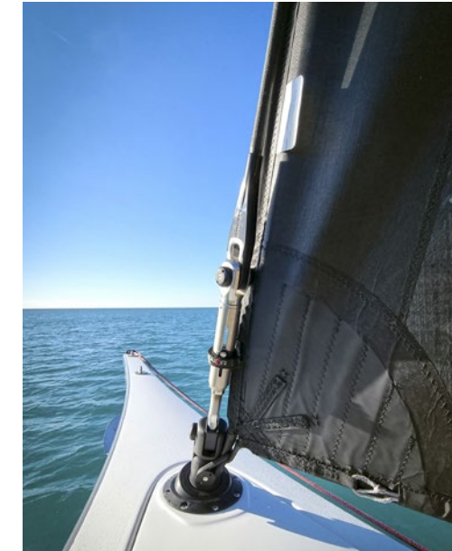
Structural torsional forestay rigged on JIBER furling unit - Photo courtesy © UBI MAIOR Italia
